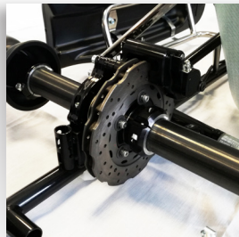
Floating rear brake disk Ø196mm
