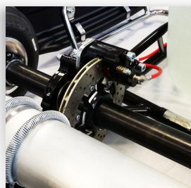
Hydraulic rear brake, ventilated disk 12mm
